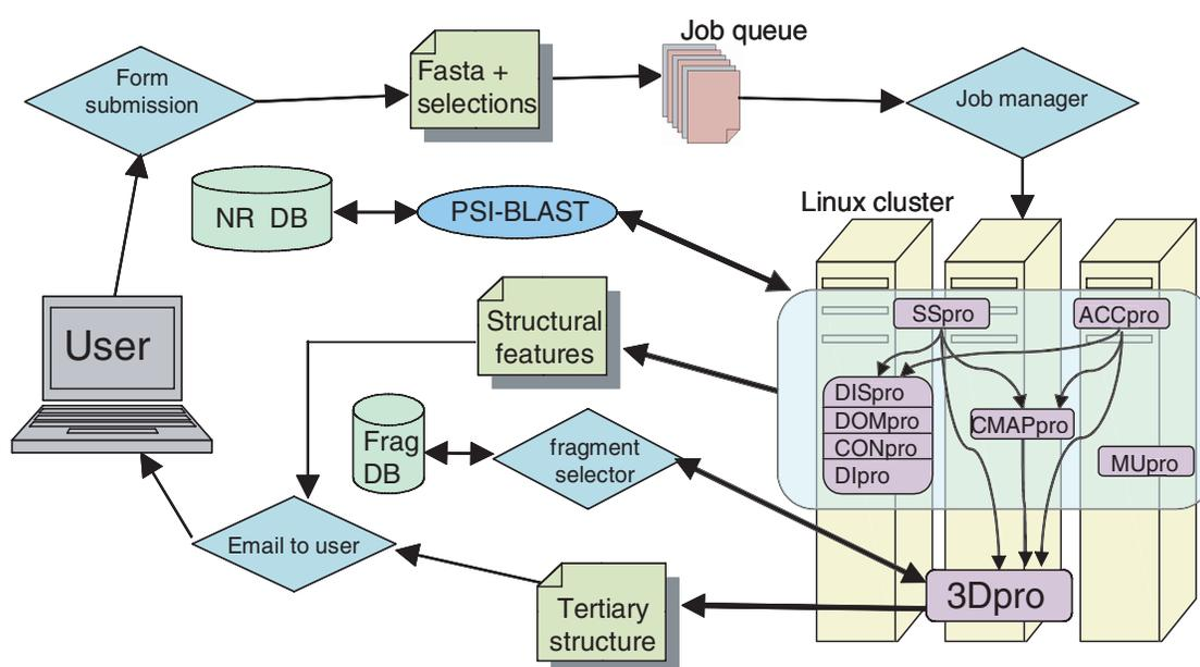
**Figure 1.** Flow diagram for the SCRATCH server. DISpro, DOMpro, CONpro and DIpro are grouped together because they have the same inputs and their outputs are not used by other predictors; however, they are standalone programs.
